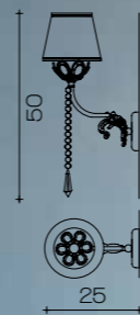
Art. 1744/A1/ORO24K H 50 cm Pø 16 cm Sp 25 cm 1 x E14 x 40W
